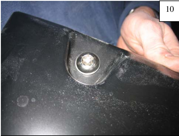
Insert one Screw/Washer assembly through each pocket hole drilled in Step 8.
