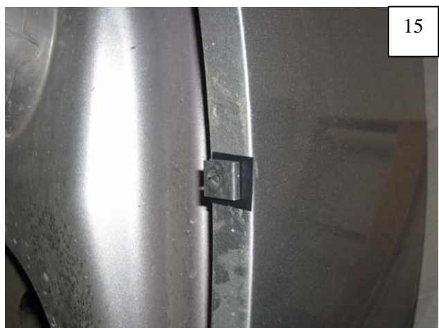
Slide a supplied "S" Clip over each black tab. Clips may need to be adjusted to align with holes in flare.
